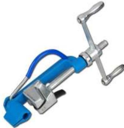
For use on band widths of 1/4" to 3/4" (.015" - .030" thickness). Strapping tool with built in cutter, spring loaded gripper lever improves ease of use.
