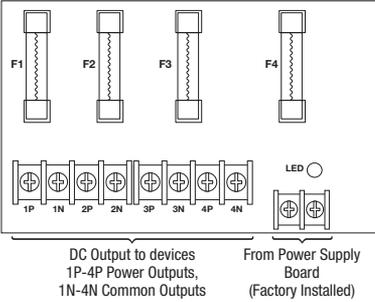
*Fig. 2b* - PD4ULCB Power Distribution Board
