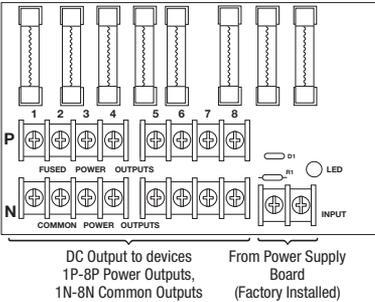
*Fig. 3b* - PD8ULCB Power Distribution Board
